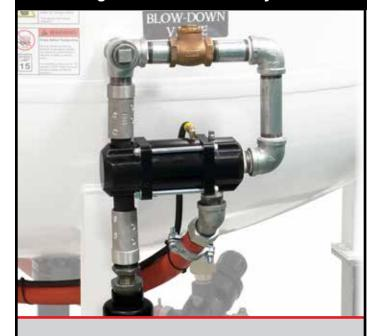
Allows you to pressurize and de-pressurize abrasive vessel with a single point palm button control.
