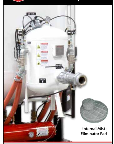
Allows airborne moisture to coalesce and drop out of the air. Water is then expelled through the drain at the bottom of the moisture separator. The drier the compressed air being used, the more trouble-free blasting will be. For added protection, consider an after cooler or air dryer, both available from Pirate Brand®.
