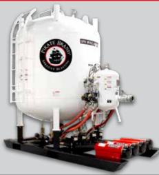
able to de-pressurize the system even when an obstruction jams in the nozzle throat or a piece of heavy equipment parks on the blast hose.
