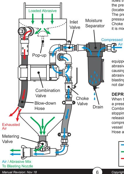
pinches the Blow-down Hose and air flows through the Combination Valve into the pressure vessel causing the Pop-up (located internally) to seal against its seat. The pressure vessel is now sealed and pressurized. Air will also continue past the Choke Valve to the Metering Valve where it is mixed with abrasive. The mixture of
